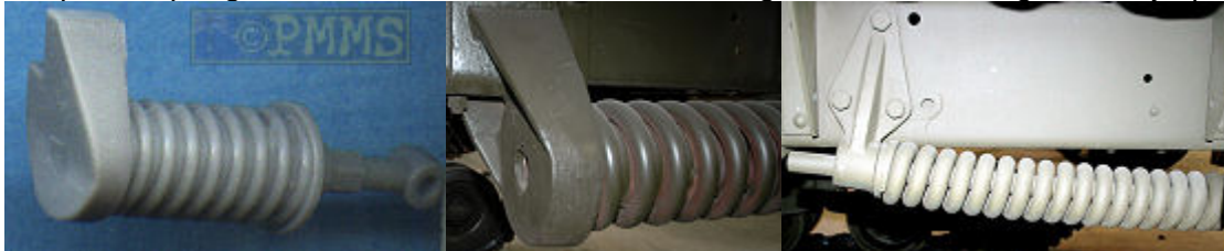
Simplified spring units could do with the end mountings reworked. Image of early spring unit (right)
