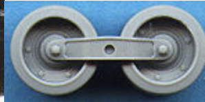
Simplified spring units could do with the end mountings reworked. Image of early spring unit (right)
